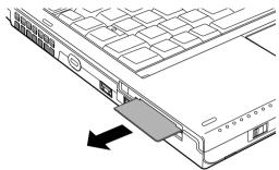
Figure 3-4 Removing a Smart Card
